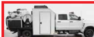
CCTV mainline inspection and vac unit : 2021 Chevy quad cab 5500 4WD : VEHICLE CAPABILITIES : Hydro Jetter 600ft at 4000 psi, 1/2 inch hose 18gpm : Vac system w/ 500 gallon debris body : Rausch Eco-Star 400 Mainline Camera System : CAMERA EQUIPMENT- Rausch L135 & KS135 : SUPPORT EQUIPMENT - Vehicle comes equipped with 1000 ft mainline cable, 2000lb lifting hoist. PRICE $195,000. CONTACT - Christiana 916-707-0067. CA (P05)
