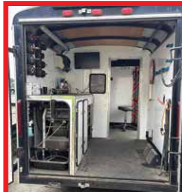
CCTV Sewer & Storm Inspection Unit : 2013 Interstate Trailer : Arias Saturn 3 CCTV Mainline Inspection System : EQUIPMENT- Pathfinder Camera Head 360 degree self cleaning lens and crawler : Electronic Control Panel (PR-3300 Series) : Multiple Wheel Sets (Various Pipe Sizes) : Inspection Cable & Reel System. SUPPORT EQUIPMENT - Unit comes equipped with exterior mounted traffic stands, internal toolbox and a Honda EU7000 Generator. PRICE $18,500 : CONTACT Christiana 916-707-0067. CA (P05)
