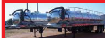
In stock, 6000- and 6300-gallon aluminum single-compartment Imperial vacuum trailers. Call Cory 800-558-2945 Ext. 426 (PBM)
