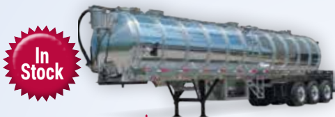
In Stock 7000 - 9000 Gal. Aluminum Tri-Axle Trailers | Air ride suspension (tri-axle), pump platform, bright finish, LED lights, Betts valves.
