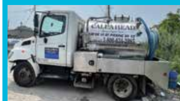
2007 HINO 185 Best Enterprises stainless steel pump truck. Tank is 1050 gallons. 700 waste, 350 water. 96 toilet paper roll tool box. Conde SDS series. PTO driven pump. $34,000.00, 1-800-634-2085 (P12)
