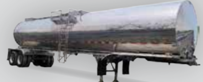
2018 9000 Gallon | 93,000 GVWR transport (aluminum tank insulated stainless steel wrapped) 6" discharge Tandem Trailer
