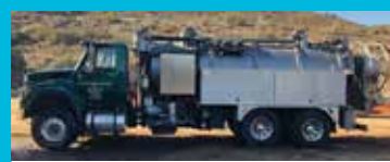
2011 ABCO Mobile Dewatering Truck - can be used as traditional pumper as well. 350 HP Maxxforce 10 motor, 1,100 foot pounds torque, 30' long 3,200-gallon tank. Dewatering filter rate 50-150 gallons per minute, automated valves. 10-wheel PDL and engine brake, air-ride seat and backup camera. Allison 3500 automatic transmission, custom automated hose reel and hydraulic rear hatch. 800 CFM Wallenstein vacuum pump. 760-532-1811. CA (P02)
