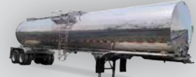
93,000 GVWR transport (aluminum tank insulated stainless steel wrapped) 6" discharge 2018 9000 Gallon Tandem Trailer
