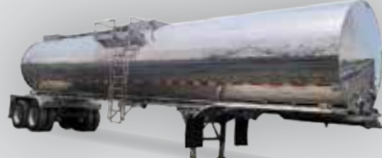
2018 9000 Gallon Tandem Trailer | 93,000 GVWR transport (aluminum tank insulated stainless steel wrapped) 6" discharge
