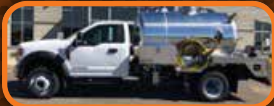
(139901) NEW Imperial 1300 U.S. gallon, portable toilet service unit mounted on a 2022 Ford F550 cab and chassis with a Masport HXL4 pump package.
