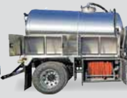
2021 Kenworth T880 CALL FOR PRICING | 20/20/46-Ultra-Shift, 200/4000/1400 aluminum decant tank, NVE 4310 blower package, strobes, cameras
