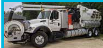
06 IH 7600 & Vactor 2100. IH SN 6J293064 & Vactor SN 2115-824RCS-18. Pre-Emission Cat C13, SN OKCB47665 with 11,200 hours on Dealer installed long block & $8,000 spent on new radiator and front of engine last year. Full opening SS rear door with hydraulic door locks and splash guard. Dual SS float ball shutoffs & SS cyclone air filter system. Roots 824 blower, factory rated @3,500 CFMs. Eight-inch boom hose with hydraulic extension to 20FT. Joystick & wireless remote boom controls. 12-volt cold weather re-circulation and air purge systems. Lakota 760, 750000 BTU boiler & 75 FT. of 1/2" hydro-excavation hose. 1,500-gallon fresh water tanks. Full range articulation hose reel with 650 FT. of 1" jetter hose. Multiple aluminum tool boxes & three tube racks. LED work lights on boom & strobe lights on truck. New drive and rear brakes August of 2020 & truck has current DOT. Asking $69,900. Call 608-790-6635, Randy. MN (P09)
