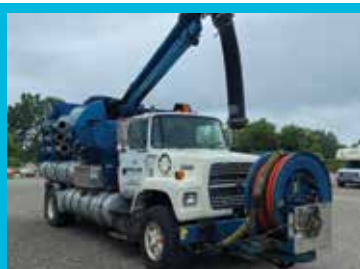
1995 Ford L 8000 Vactor 2100 8.3L Cummins. 61,409 miles single axle 5-speed manual transmission. Fan unit 3.9L John Deer w/6526 hours. 10-yard debris body with pump off system. 1,300 gallons fresh water, 600-foot hose reel and cold weather recirculator. $25,000 obo. Any questions call Steve 248-345-5960. (P10)
