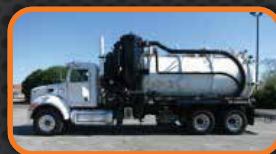
(1121C) Pre-owned 3,600 U.S. gallon, carbon steel, Cusco Omni-Vac. D.O.T. 407/412 Certified. Mounted on a 2012 Peterbilt 348 cab & chassis.
