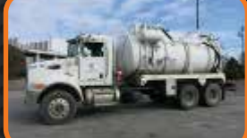
(9277C) 2013 Peterbilt 348 cab & chassis with a Presvac 3,200 U.S. gal., C/S, D.O.T. 412, dump type, vacuum tank and a Presvac PV750 pump.
