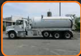
(7896C) 2001 Freightliner cab & chassis with a Keith Huber 4,000 gallon c/s full open rear door dump unit.
