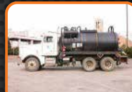
(6625C) 1997 Peterbilt 378 cab & chassis with a Presvac 3,000 U.S. gallon, C/S, vacuum tank & Masport HXL15WV water cooled pump.
