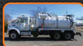
(0200V) 2011 Peterbilt 348 cab & chassis with a Presvac 3,200 U.S. gallon, C/S, D.O.T. 412, dump type, Vacuum tank and a Presvac PV750 pump.
