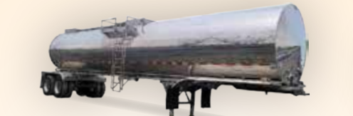
2018 9000 Gallon Tandem Trailer | 93,000 GVWR transport (aluminum tank insulated stainless steel wrapped) 6" discharge
