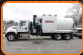
(033R) VACALL ALLVAC AVRB-18 yard debris body mounted on a 2014 Freightliner 114SD cab and chassis.
