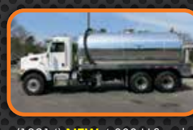
(13914) NEW 4,000 U.S. gal., aluminum, vacuum-pressure tank mounted on a 2021 Peterbilt 348 cab & chassis with NVE Challenger 887 fan-cooled vacuum pump.
