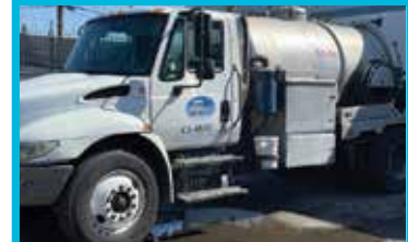
2005 International DT466 , 269k miles, automatic Allison transmission, Keith Huber aluminum 1,750-gallon tank (350-gal fresh water, 1,400-gal waste). Dual-side service. HXL 75 Masport pump. Onboard 1100 psi pumptec pressure washer with dual 50' hose reels. Owned since brand new. Serviced every 8,000 miles. May not look pretty but a great everyday work truck. Gary 818-266-1626. CA (P04)
