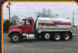
(6025V) 2005 MACK CV713 cab & chassis with a Presvac 4,200 gallon 200 water, 4000 waste tank and Jurup pump
