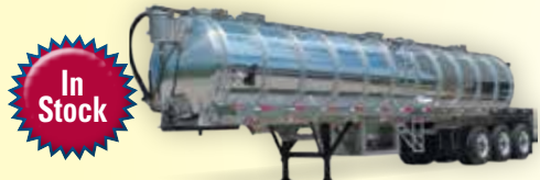
7000 - 9000 Gal. Aluminum Tri-Axle Trailers | Air ride suspension (tri-axle), pump platform, bright finish, LED lights, Betts valves.
