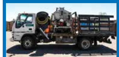
Chassis 2007 Isuzu NRR Service Truck. 19,500lbs with a 132" wheelbase. Tank is Progress aluminum with 200-gallon fresh water capacity and 400-gallon waste capacity installed by FMI Portland in June of 2014 along with a Honda Direct Drive. Can haul 6 toilets: 4 with the lift gate up, 2 on the lift gate. This truck was a flatbed originally and we purchased, installed tank, liftgate, and hitch in 2014 for an event vehicle. We wanted an NRR for the larger breaks, wheels, and lower rear ratio to be able to pull trailers and still service up to 40 toilets on a smaller route. We are upgrading our fleet to newer models. Maintenance records are available upon request. $25,000. Please contact kimi@portapros.com or call/text 541-212-3175 for more information. ID (P12)
