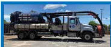
2015 Ex-Municipal Vactor 2100 Plus with PD Blower mounted on a Freightliner chassis. 12-yard debris tank, 1,500-gallon water, 80 gpm @ 2,500 psi with 600' 1" rodder hose. HydroX package, Bellypack Wireless remote, debris body flush out, and low pressure 50' handgun. Only 21,700 miles and 4,100 hrs. Call Richard for pricing 803-609-9140. (P11)
