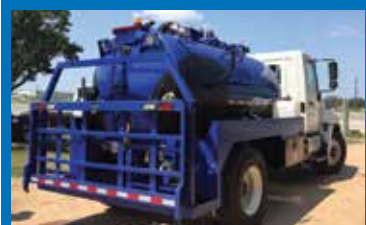
(7295C) 2001 International 4700 cab & chassis with a Transway 2,400 U.S. gal. , carbon steel, dump type vacuum tank with a Fruitland RDF500 vacuum pump.
