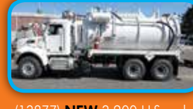
(13877) NEW 3,200 U.S. gal. , carbon steel, D.O.T. certified 412 vacuum tank; dump type with full open rear door and a Presvac PVB 750 vacuum-pressure pump installed on a 2021 Peterbilt 348 cab & chassis.
