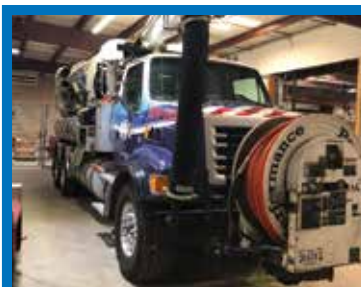
2007 Vactor 2112-PD - multi-flow, accumulator, 15" roots blower 80-2,000 PSI water pump, flat rear door. Curb side and road side, pipe fold down racks. New boom inner, extension tube and 90. Both suction hoses 8" new and plate at tank new. New cyclone separator 2019 and final filter housing. Debris tank sand-blasted and marine coated with new rear door gasket in 2019 and new decant butterfly valve. Blower serviced at dealer 2019. Well-maintained truck ready for work. Ex municipal truck out of South Carolina. Miles 173,750, total truck hours 13,102.1 as of 6/24/2020. $175,000. 757-490-7050. VA (P09)
