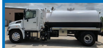
2020 Hino 338 , 260hp engine, Allison automatic transmission, trailer hookups, 2,500-gallon steel vac tank, Jurop 260 vac pump, 36" rear hatch, (2) 4" suction parts, 36" toolbox. ... $108,500
