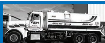
1997 Peterbilt 379 , C-12 engine, 240k miles, 3,600-gallon PikRite vacuum tank, 750 Presvac vacuum pump. Works daily. .... $50,000 OBO
