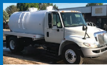
2013 International 4300 , under CDL. DT466 diesel, auto., 130k miles. NEW 1,800-gallon steel vacuum tank with Masport pump.
