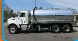
(13865) New 4,000 U.S. gal., aluminum, vacuum-pressure tank mounted on a 2020 Peterbilt 348 cab & chassis with NVE Challenger 887 fan cooled vacuum pump.
