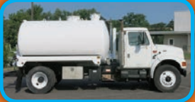
(7295C) 2001 International 4700 cab & chassis with a Transway 2,400 U.S. gal., carbon steel, dump type vacuum tank with a Fruitland RDF500 vacuum pump.
