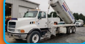
(3408C) Pre-owned Keith Huber Dominator , 4,000 U.S. gal., two compartment, dump type unit, with a Becker 440 vacuum pump package. Mounted on a 1999 Sterling cab & chassis.
