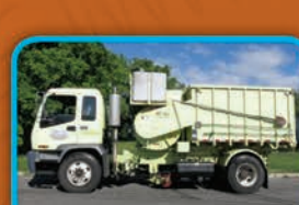
(044R) 2004 GMC T7500 dual steer cab & chassis with a VACALL LV10SC single sweep street sweeper.
