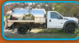
(4246V) 2012 Ford F550 cab & chassis with an Imperial 1,100 U.S. gallons, 3 compartment 150/600/350 Aluminum portable toilet service unit, with a Masport HXL4 vacuum pump.
