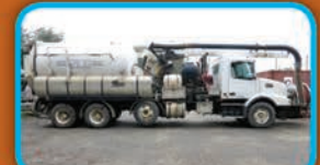
(5903C) 2007 Volvo VHD cab & chassis with a Vector 2115 combination Vacuum Loader and High Pressure sewer cleaning system.
