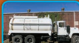
(8463C) 1983 Mack R686ST cab & chassis with a Presvac 3,200 U.S. gal., carbon steel vacuum tank with Masport H15WV vacuum pump.
