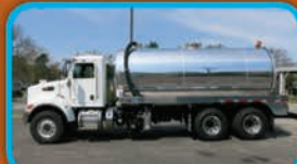
(13822) New 4,000 U.S. gal., aluminum, vacuum-pressure tank. Mounted on a 2020 Peterbilt 348 cab & chassis with a NVE 866 fan cooled pump.
