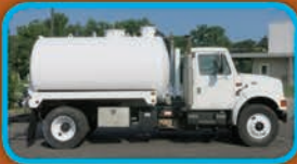
(7295C) 2001 International 4700 cab & chassis with a Transway 2,400 U.S. gallon, carbon steel, dump type vacuum tank with a Fruitland RDF500 vacuum pump.
