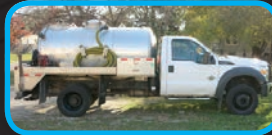
(4246V) 2012 Ford F550 cab & chassis with an Imperial 1,100 U.S. gallons, 3 compartment 150/600/350 Aluminum portable toilet service unit, with a Masport HXL4 vacuum pump.
