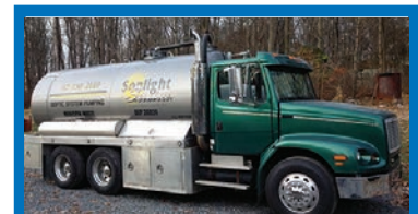
2004 Freightliner FL112 , 370hp, Eaton 10-speed transmission, 192" WB, 426k miles. 3,600-gallon tank, Jurup LC420 water-cooled pump, 52k GVW. See-level gauge, 100 ft. 4-inch hose reel, General Pump 10gpm/3,000 psi pressure washer/jetter with 100-gallon freshwater tank. Very fuel efficient truck! Email for more photos. .... $39,000 OBO
