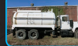
(8463C) 1983 Mack R686ST cab & chassis with a Presvac 3,200 U.S. gal., carbon steel vacuum tank with Masport H15WV vacuum pump.
