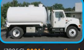
(7295C) 2001 International 4700 cab & chassis with a Transway 2,400 U.S. gallon, carbon steel, dump type vacuum tank with a Fruitland RDF500 vacuum pump.
