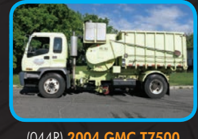
(044R) 2004 GMC T7500 Dual steer cab & chassis with a VACALL LV105C single sweep street sweeper.
