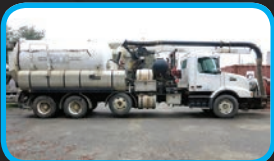
(5903C) 2007 Volvo VHD cab & chassis with a Vactor 2115 combination Vacuum Loader and High Pressure sewer cleaning system.
