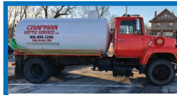
1986 Ford 8000 , 3208 Cat diesel, 10-speed, 32k GVW. 2,200-gallon steel tank (lined inside), 6" heated discharge valve, 4" heated inlet valve. Masport water-cooled pump (230cfm), 70% rear tires, 15% steer tires. .... $10,900
