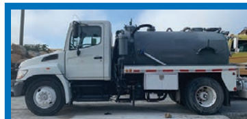
2007 Hino 268A , 275k miles, auto. transmission, a/c, cruise. 1,500-gallon tank (1,100 waste, 400 freshwater), Masport vac pump. .... $30,000
