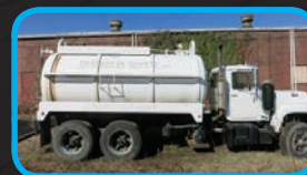
(8463C) 1983 Mack R686ST cab & chassis with a Presvac 3,200 U.S. gal., carbon steel vacuum tank with Masport H15WW vacuum pump.
