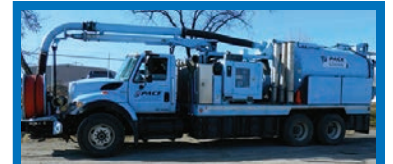
2008 International Vac-Con combo unit for sale. 1,500-gallon water tank, 2,000-gallon debris tank. 60gpm/2,000psi pump, 1" x 800' hose reel. 8,150 hrs, 61k miles. .... $60,000
