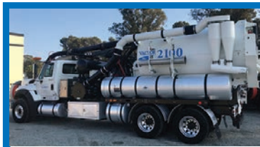
2013 Vactor 2100PD, International 7600 . 12-yard debris, 1,300-gallon water, 80gpm/2,500psi. Vacuum relief system, 60" dump-height, load limit alarm, centrifugal separators. 180-degree 5x5 boom. Cold-weather recirculator, jet rodder system accumulator, hydro-excavation kit, 4-way camera system. Please call for price. ID# V032-C
