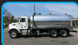
(13822) New 4,000 U.S. gal., aluminum, vacuum-pressure tank. Mounted on a 2020 Peterbilt 348 cab & chassis with a NVE 866 fan cooled pump.
