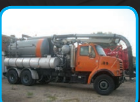
(2775V) 1999 Sterling chassis with a Vector 2110 combination vacuum loader and high pressure sewer cleaning system.
