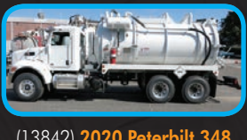
(13842) 2020 Peterbilt 348 cab & chassis with with PX9—350 HP & automatic transmission. Presvac 3,200 U.S. gallon, carbon steel, full open rear door, dump type unit with a Presvac PV750 vacuum pump.
