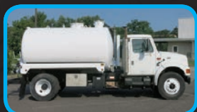
(7295C) 2001 International 4700 cab & chassis with a Transway 2,400 U.S. gallon, carbon steel, dump type vacuum tank with a Fruitland RDF500 vacuum pump.
