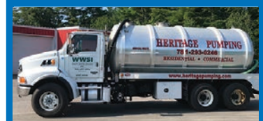
2007 Sterling LT9513 , 405,833 miles. Mercedes Benz 4000 - 410hp. Eaton-Fuller 8LL transmission. 2008 Progress 4,800-gallon aluminum tank. NVE 866 vacuum pump. Water jetter. Heated valves. .... $65,000
