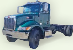
2019 Peterbilt 337 IN STOCK 300HP, Allison Auto, 33GVWR de-rated to 26GVWR ready for tank
