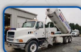
(3408C) Pre-owned Keith Huber Dominator , 4,000 U.S. gal., two compartment, dump type unit, with a Becker 440 vacuum pump package. Mounted on a 1999 Sterling cab & chassis.
