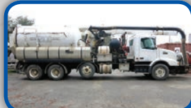
(5903C) 2007 Volvo VHD cab & chassis with a Vector 2115 combination Vacuum Loader and High Pressure sewer cleaning system.
