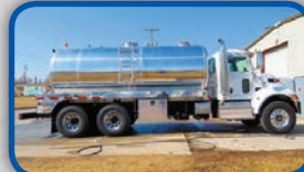
(13789) New 4,000 U.S. gal., aluminum, vacuum-pressure tank. Mounted on a 2019 Peterbilt 348 cab & chassis with a NVE 866 fan cooled pump.
