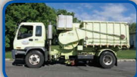
(044R) 2004 GMC T7500 Dual steer cab & chassis with a VACALL LV10SC single sweep street sweeper.
