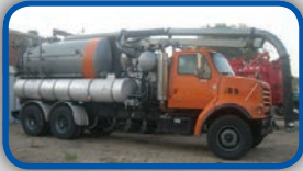
(2775V) 1999 Sterling cab & chassis with a Vector 2110 combination vacuum loader and high pressure sewer cleaning system.
