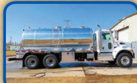
(13789) New 4,000 U.S. gal., aluminum, vacuum-pressure tank. Mounted on a 2019 Peterbilt 348 cab & chassis with a NVE 866 fan cooled pump.
