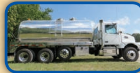
(13796V) New 4,800 U.S. gal., aluminum, vacuum-pressure tank mounted on a 2019 Volvo VHD tri-axle cab & chassis with an NVE 866 fan cooled vacuum pump.
