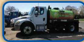
(4468C) Pre-owned 1,500 U.S. gal., carbon steel, vacuum pressure tank. Mounted on Freightliner M-2 cab and chassis with a Masport HXL400WV vacuum pressure pump.
