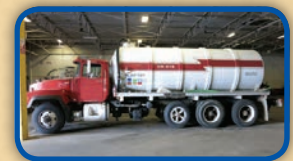
(3130V) 1997 Mack RD688S Tri-Axle cab & chassis with a 4,500 gal. aluminum vacuum tank and Wittig RFL100 pump package.
