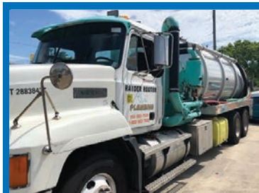
1995 Mack: This truck has a 4,000-gallon aluminum tank and jetter with 300-gallon freshwater tank. It needs a transmission and clutch. .... $19,000
