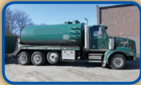
(7347V) 2005 Western Star 4900 Tri-Axle cab & chassis with a 5,000 carbon steel vacuum tank & Masport HXL20WV pump package.
