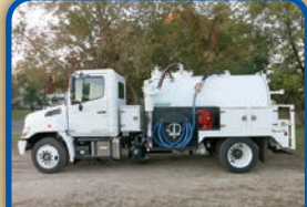
(13762) 2018 Hino 268A cab & chassis 25,950 GVW with a new 1600 gal., potable toilet service unit.
