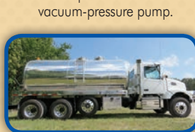
(13796V) New 4,800 U.S. gal., aluminum, vacuum-pressure tank mounted on a 2019 Volvo VHD tri-axle cab & chassis with an NVE 866 fan cooled vacuum pump.
