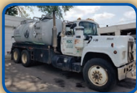
(1165C) 1984 Mack R686ST with a 1999 Keith Huber Dominator 3000 carbon steel, dump type, DOT, vacuum tank unit.
