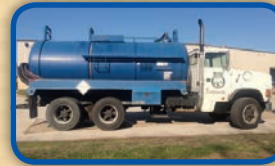
(1829V) 1997 Ford cab and chassis with a 3,500 U.S. gal., carbon steel, D.O.T. certified vacuum tank; dump type. With full open rear door and a Masport HXL400WV vacuum-pressure pump.
