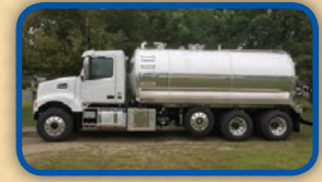
(13801V) NEW 5,000 U.S. gal., aluminum, vacuum-pressure tank mounted on a 2019 Volvo VHD tri-axle cab & chassis with an NVE 4310 PD blower package.
