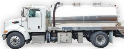
2019 Peterbilt 337 NEW | 330HP, auto, 2800 gal. aluminum tank, NVE 4310 blower package.
