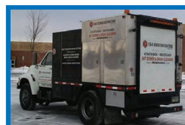
1995 Ford F800 Jet Truck. 7.8L Ford diesel. Allison automatic transmission. Sewer Equipment Co. 800 Series jetter. 1,500-gallon water tank, rotating hose reel. Hydraulic and water pump both have been rebuilt. 60 gallon per minute pump. Truck runs 1" and 1/2" hose.
