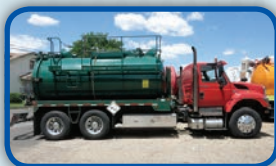
(3241V) 2011 International 7500 with a Presvac 3,200 c/s, DOT. Dump type vacuum tank and Presvac PV750 pump.
