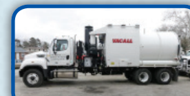
(035R) VACALL ALLVAC AVR-B 18 yard debris body mounted on a 2015 Freightliner 114SD cab and chassis
