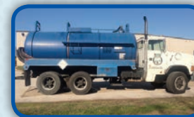
(1829V) 1997 Ford cab and chassis with a 3,500 U.S. gal., carbon steel, D.O.T. certified vacuum tank; dump type. With full open rear door and a Masport HXL400WW vacuum-pressure pump.
