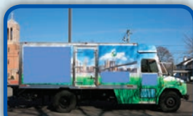
(4101V) 2004 Freightliner FL70 low entry cab with a van body and lift gate with a 1200 gal. unit.
