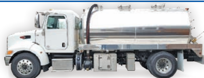
2018 Peterbilt 337 330HP, auto, 2800 gal. aluminum tank, New NVE 4310 blower package.
