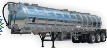
7000 - 9000 Gal. Aluminum | Air ride suspension (tri-axle), pump platform, Tri-Axle Trailers bright finish, LED lights, Betts valves.
