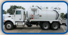
(034R) Pre-owned 3,200 U.S. gallon, carbon steel, D.O.T. certified 412 vacuum tank; dump type with full open rear door and a Presvac PVB 750 vacuum-pressure pump installed on a 2014 Peterbilt 348 cab and chassis.
