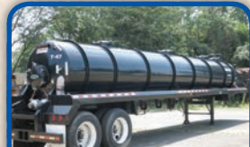
(3901C) 2012 Dragon 5,460 U.S. gallon, Steel, vacuum tank trailer.
