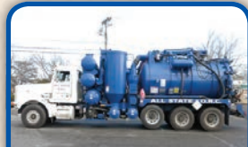
(602SV) 1999 Peterbilt 378 triaxle with a Presvac Power-vac 5300 , 3,250 carbon steel, DOT, industrial vacuum loader
