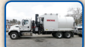
(035R) VACALL ALLVAC AVRB - 18 yard debris body mounted on a 2015 Freightliner 114SD cab and chassis
