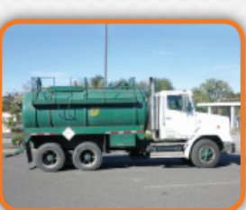
(9382V) 1989 Freightliner with a Presvac 3,500 gallon, carbon steel vacuum tank and a PV750 vacuum pump.
