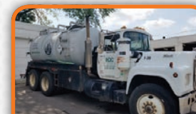
(1165C) 1984 Mack R686ST with a 1999 Keith Huber Dominator 3000 carbon steel, dump type, DOT, vacuum tank unit.
