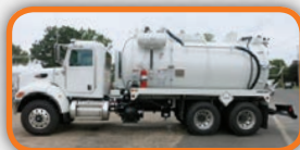
(034R) Pre-owned 3,200 U.S. gallon, carbon steel, D.O.T. certified 412 vacuum tank; dump type with full open rear door and a Presvac PVB 750 vacuum-pressure pump installed on a 2014 Peterbilt 348 cab and chassis.
