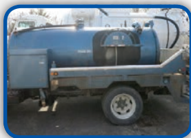
(602SV) 2002 Keith Huber portable toilet service tank 700 waste & 350 water.
