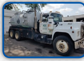
(1165C) 1984 Mack R686ST with a 1999 Keith Huber Dominator 3000 carbon steel, dump type, DOT, vacuum tank unit.
