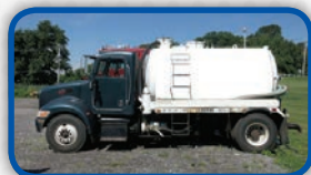
(8481C) Pre-owned 2004 Peterbilt 335 cab and chassis with a 2,500 U.S. gallon carbon steel vacuum tank. Complete with a Transway TS1500 vacuum pump package.
