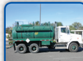
(9382V) 1989 Freightliner with a Presvac 3,500 gallon, carbon steel vacuum tank and a PV750 vacuum pump.
