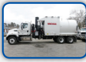
(035R) VACALL ALLVAC AVR8- 18 yard debris body mounted on a 2015 Freightliner 114SD cab and chassis
