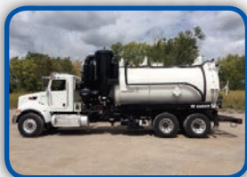
(6131C) Pre-owned 3,600 U.S. gallon, carbon steel, Cusco Omni-Vac. D.O.T. 407/412 Certified. Mounted on a 2013 Peterbilt 348 cab & chassis.
