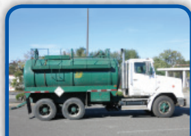
(9382V) 1989 Freightliner with a Presvac 3,500 gallon, carbon steel vacuum tank and a PV750 vacuum pump.
