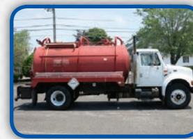
(0529V) Pre-owned 2,300 U.S. gallon, carbon steel, D.O.T. certified, vacuum pressure tank. Mounted on 2002 International PVB 750 vacuum pressure pump.
