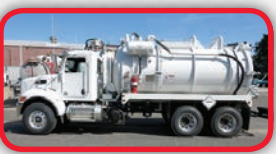
(13671 A-C) NEW 3,200 U.S. gallon, carbon steel, D.O.T. certified 412 vacuum tank; dump type with full open rear door and a Presvac PVB 750 vacuum-pressure pump installed on a 2017 Peterbilt 348 cab and chassis.
