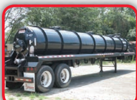
(3901C) 2012 Dragon 5,460 U.S. gallon, Steel, vacuum tank trailer.
