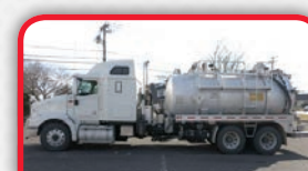
(2757C) Pre-owned 3,180 gallon, two compartment, aluminum, D.O.T. 407/412 vacuum tank, with a NVE Challenger 357 pump package. Installed on a 2007 International.
