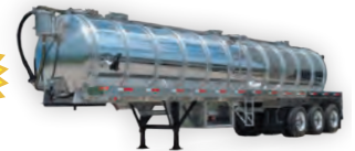
8000 & 9000 Gal. Aluminum Tri-Axle Trailers, Air ride suspension (tri-axle), pump platform, bright finish, LED lights, Betts valves. IN STOCK
