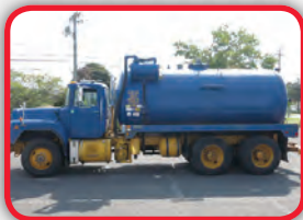
(4987C) Pre-owned 1999 Mack RB688S with a 4,000 gallon, carbon steel vacuum tank and Masport HXL15WV pump package
