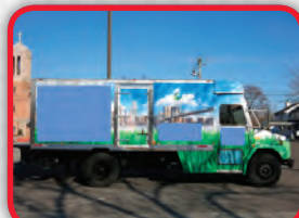
(4101V) 2004 Freightliner FL70 low entry cab with a van body and lift gate with a 1200 gallon unit.
