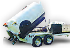
2016 Dodge 5500 Diesel (4 X 4), Auto, 1200 aluminum RVT, NVE 304 hydraulic drive pump package, DC10, two unit carrier.
