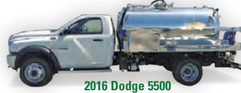
2016 Dodge 5500 Diesel (4 X 4), Auto, 1200 aluminum RVT, NVE 304 hydraulic drive pump package, DC10, two unit carrier.
