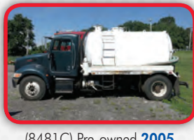
(8481C) Pre-owned 2005 Peterbilt 335 cab and chassis with a 2500 U.S. gallon, carbon steel vacuum tank complete with Fruitland RCF500 vacuum pump package
