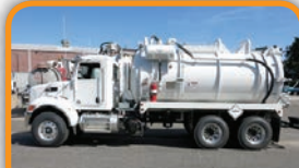
(13671 A-C) NEW 3,200 U.S. gallon, carbon steel, D.O.T. certified 412 vacuum tank; dump type with full open rear door and a Presvac PVB 750 vacuum-pressure pump installed on a 2016 Peterbilt 348 cab and chassis.
