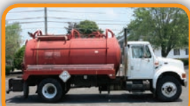
(0529V) Pre-owned 2,300 U.S. gallon, carbon steel, D.O.T. certified, vacuum pressure tank. Mounted on 2002 International cab and chassis with a Presvac PVB 750 vacuum pressure pump.
