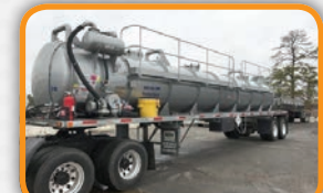
(5002C) Pre-owned 2016 Presvac , 5,500 U.S. gallon, Carbon Steel, D.O.T. 412 (A.S.M.E.) vacuum tanker.
