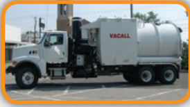
(4792C) Vacall AllVac AVR8 - 18 yard debris body mounted on a 2009 Sterling LT9500 cab and chassis.
