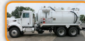
(034R) Pre-owned 3,200 U.S. gallon, carbon steel, D.O.T. certified 412 vacuum tank; dump type with full open rear door and a Presvac PVB 750 vacuum-pressure pump installed on a 2014 Peterbilt 348 cab and chassis.
