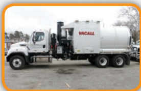
(9116C) Vacall AllVac AVR B - 18 yard debris body mounted on a 2014 Freightliner 114SD cab and chassis.
