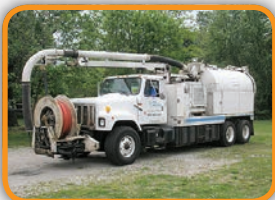
(3918C) VacCon industrial machine mounted on a pre-owned 1999 International cab and chassis.
