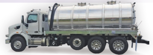
2017 567 Peterbilt 10-speed, 485 HP, tri-axle, aluminum wheels, 5,000 gal. tank, NVE 866 "Max" package liquid cooled, all air, loaded
