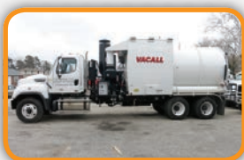
(9116C) Vacall AllVac AVR B - 18 yard debris body mounted on a 2014 Freightliner 114SD cab and chassis.
