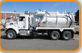
(13671 A-C) NEW 3,200 U.S. gallon, carbon steel, D.O.T. certified 412 vacuum tank; dump type with full open rear door and a Presvac PVB 750 vacuum-pressure pump installed on a 2016 Peterbilt 348 cab and chassis.
