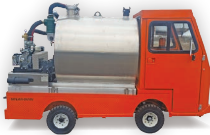
2017 Taylor-Dunn 500 gal. tank, NVE 866 pump package
