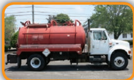
(0529V) Pre-owned 2,300 U.S. gallon, carbon steel, D.O.T. certified, vacuum pressure tank. Mounted on 2002 International cab and chassis with a Presvac PVB 750 vacuum pressure pump.
