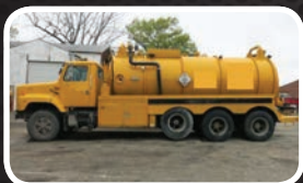
(6246C) 1992 International 2654 with a 4000 gallon, carbon steel unit.
