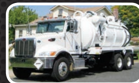
(13887A-E) 2015 Peterbilt 348, cab and chassis with a New 3,200 U.S. gal., carbon steel, D.O.T. certified 407/412 vacuum tank; dump type with full open rear door and a Presvac PVB 750 vacuum-pressure pump.
