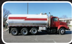
(9982V) 2000 International 2674 triaxle with 4000 waste—200 water and Wittig RFL100 vacuum pump and Harben jet pump system.
