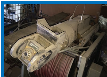
Envirosight Rover System: RA200 reel with 450' cable s/n 0361082. New termination, CCU with new cards, 6,335 hrs. S/N 0161945. Rover 125 and Rover 225. Both crawlers have new seals and lift was refurbished. Lots of extra wheels. .... $15,000 USD
