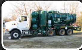
(5176C) 2006 Sterling LT9500 tri-axle with a Presvac Powervac 5300 , 3,000 gallon carbon steel High Dump with a Hibon 5300 CFM Blower DOT 407/412.
