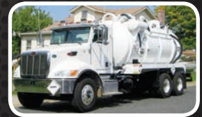
(13887A-E) 2015 Peterbilt 348, cab and chassis with a New 3,200 U.S. gal., carbon steel, D.O.T. certified 407/412 vacuum tank; dump type with full open rear door and a Presvac PVB 750 vacuum-pressure pump.
