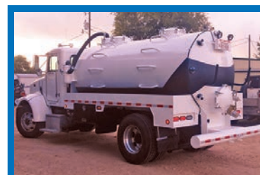
(13670V) New 4,000 U.S. gallon, aluminum, vacuum-pressure tank. Mounted on 2016 Peterbilt 348 cab and chassis with a Masport HXL400VV vacuum pressure pump package.
