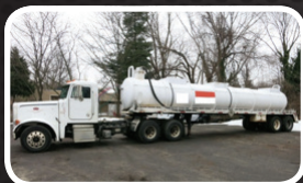
(1193C) 2002 Peterbilt 379 tractor with Wittig RFL100 pump package – Presvac 5,460 C/S vacuum tank trailer.
