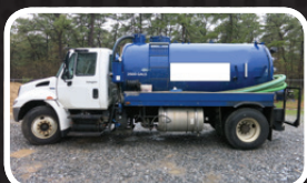
(1537C) 2008 International 4300 with 2,500 C/S vacuum tank unit and Masport pump with wash down type system.
