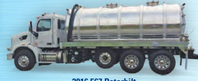
2016 567 Peterbilt 10-speed, 485 HP, tri-axle, aluminum wheels, 5,000 gallon tank, NVE 866 "Max" package liquid cooled, all air, loaded
