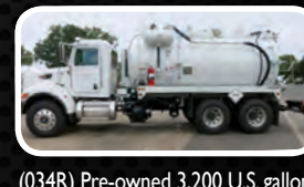
(034R) Pre-owned 3,200 U.S. gallon, carbon steel, D.O.T. certified 412 vacuum tank; dump type with full open rear door and a Presvac PVB 750 vacuum-pressure pump installed on a 2014 Peterbilt 348 cab and chassis.
