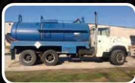
(1829V) 1996 Ford with a Presvac 3500 gallon, carbon steel, DOT vacuum tank with a Masport pump.
