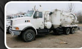
(3378V) 1999 Sterling with a 3,200 gallon Cusco Master Vac high dump unit.
