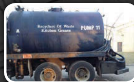
(0003V) 3,000 U.S. gallon, carbon steel vacuum tank unit, with drum holder behind cab
