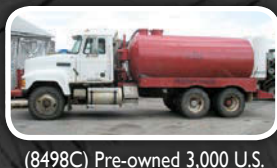
(8498C) Pre-owned 3,000 U.S. gallon, carbon steel vacuum tank; with a Masport H75W vacuum-pressure pump installed on a 2000 Mack CH613 cab and chassis.
