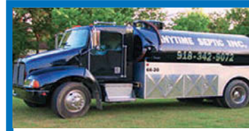
1999 Kenworth T-300: Rebuilt 3126 CAT motor & 6-speed Eaton transmission, brand-new clutch. 2,500-gallon tank 5/16" thick. 2014 model new Jurup PN84, remote-control valve.
