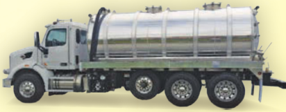
2016 567 Peterbilt 10-speed, 485 HP, tri-axle, aluminum wheels, 5,000 gallon tank, NVE 866 "Max" package liquid cooled, all air, loaded
