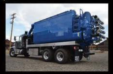
**2015 PETE** AIR MOVER WET/DRY; 17 CU YD DEBRIS BODY: 5,250 CFM. 28" Hg; SLUDGE PUMP & MORE
