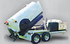
Self Contained Unit 600 gallon steel tank, 33.5 HP Kubota diesel engine (choice of pumps), 200 gallon poly tank, 6 gpm 3,000 psi jetter.
