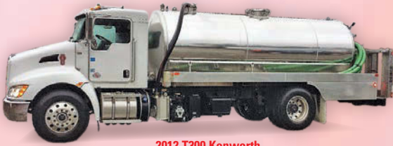
2012 T300 Kenworth 21,000 miles, 330HP, Allison auto, 200/2800 aluminum tank, NVE 607 pump package, gas powered jetter system
