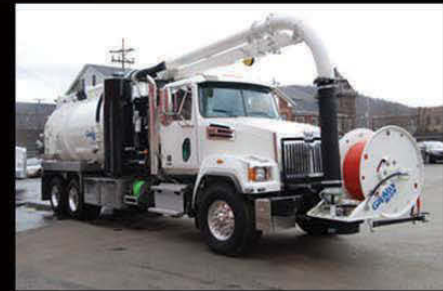
MC1510-0180 COMBO JETVAC WET-ONLY; 2014 WESTERN STAR; 1,500 GALLON STAINLESS STEEL WATER TANK; 10 CU YD DEBRIS BODY; TRASH PUMP & MORE!
