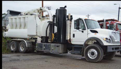
TRADE 140 HV55 HydroVAX 40,223 MILES; 5,940 ENGINE HOURS; 1,429 BLOWER HOURS; RECIRC/GLYCOL SYSTEMS; WATER BURNER; HEATED BOX AND MORE!
