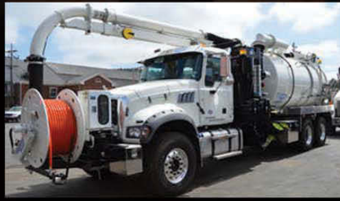
MC1510-0181 COMBO JETVAC WET-ONLY; 2014 MACK 1500 GALLON STAINLESS STEEL WATER TANK; 10 CU YD DEBRIS BODY; 26' BOOM & MORE
