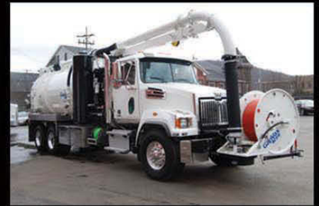
MC1510-0180 COMBO JETVAC WET-ONLY; 2014 WESTERN STAR; 1500 GALLON STAINLESS STEEL WATER TANK; 10 CU YD DEBRIS BODY; TRASH PUMP & MORE!
