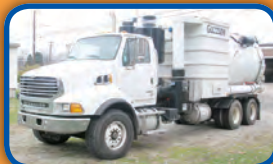
(018R) 2008 Sterling with a Guzzler Wet/Dry Industrial Vacuum Loader, 18 yard debris body, Dump type, Carbon Steel vacuum tank.
