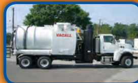
(014R) VACALL ALLVAC AVR-18 yard debris body mounted on a 2009 Sterling LT9500 cab and chassis
