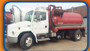
(4427V) Pre-Owned 2002 Freightliner FL70 cab and chassis with a 2,300 U.S. Gallon carbon steel vacuum tank. Complete with a Moro Vacuum pump package.
