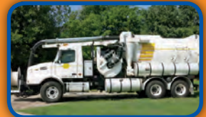
(3483C) 2006 Volvo Cab & Chassis with a Vector 2110 combination Vacuum Loader and High Pressure sewer cleaning system. "Work Ready"
