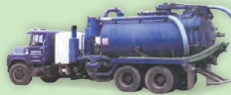
1989 Mack DM 20/44, 300 HP, 8 spd, Hibon blower, Presvac 3200 gal steel tank with dump, 300 gal wash tank and reel
