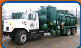
(2433V) 2002 Navistar International cab and chassis with a Powervac 5300 , 16 cubic yard, 3,250 U.S. gallons, Carbon Steel, vacuum tanker w/ Hibon PD blower.
