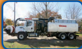
(027R) 2014 Freightliner 108 SD with a VacAll AJV1215 ; 12 yard debris body, 1500 gallons water, Combination vacuum / jetting unit.
