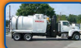
(014R) VACALL ALLVAC AVRB- 18 yard debris body mounted on a 2009 Sterling LT9500 cab and chassis
