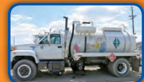
(6615V) Presvac 2,300 U.S. gallon, Carbon Steel with a Masport H15W vacuum pump installed on a 1993 GMC Kodiak cab and chassis.
